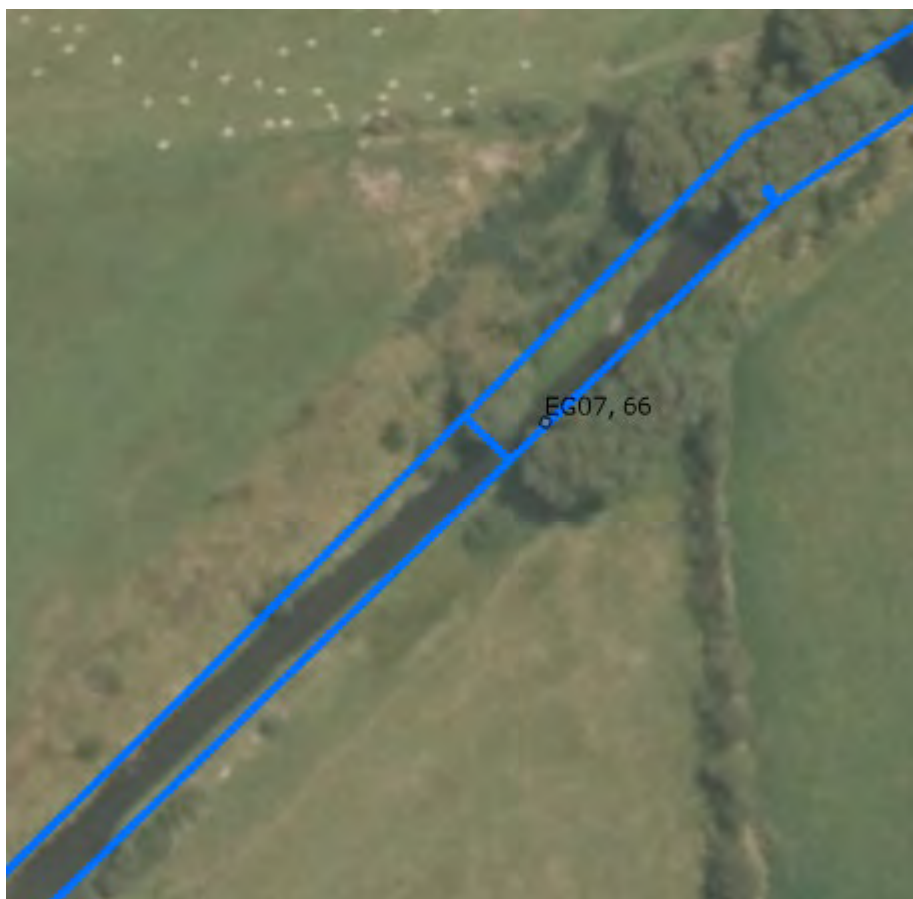
Figure 5 – Examples of splitting the stream into two different polygons consistent with the change in habitat type around the riparian margin.
