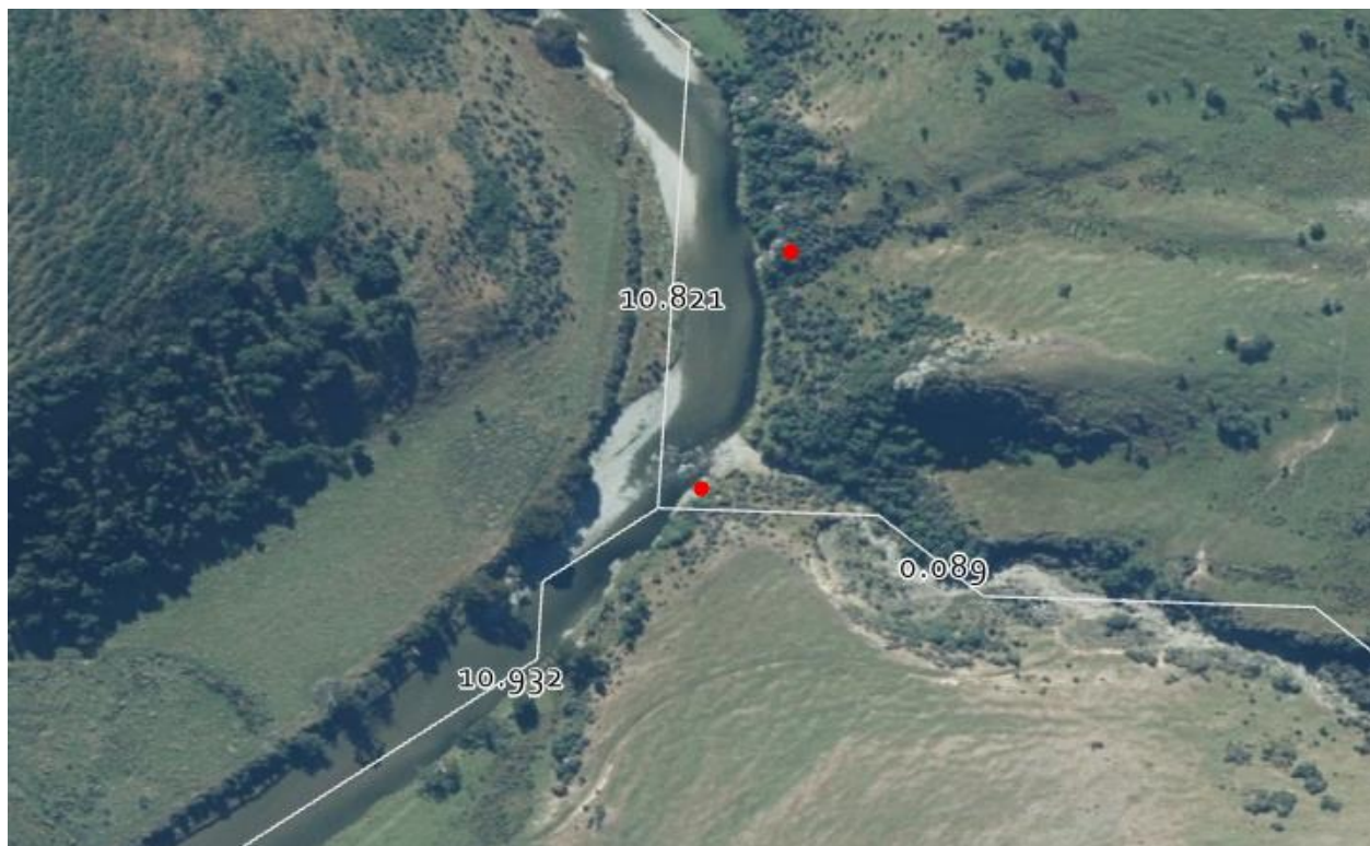
Figure 4: Screenshot showing two redds marked in red, overlaid with waterway shapefiles labelled with their modelled flow. Note that the more southern redd would have been incorrectly allocated to the very small tributary below it in earlier models.
