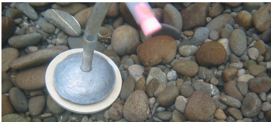
Figure 8b. An IGDO probe in place in Silverstream. Hemi-spherical lead weights were added to weight the probes as a precaution against the probes washing out of the redds during freshes. The terminal bung can be seen which prevents surface water contaminating the intragravel water.
