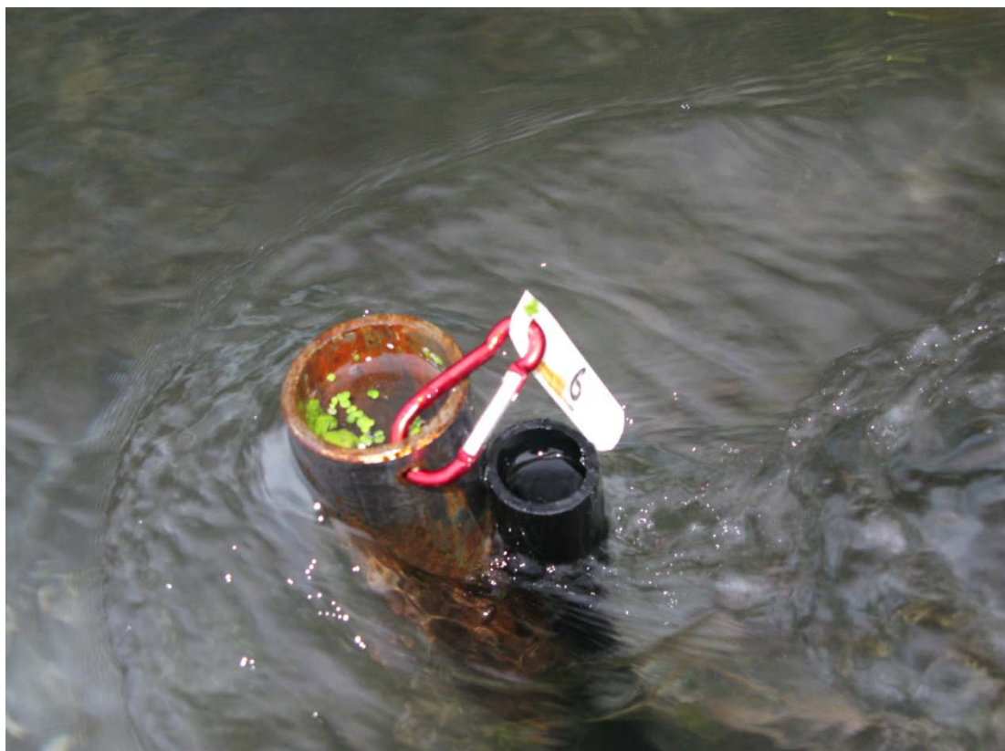
Figure 10. A deeply-placed redd at Silverstream, where the \Delta H component could be directly observed. The parameter \Delta H is the difference in water level between the upwelling in the steel standpipe and the water surface in the black PVC stilling well.
