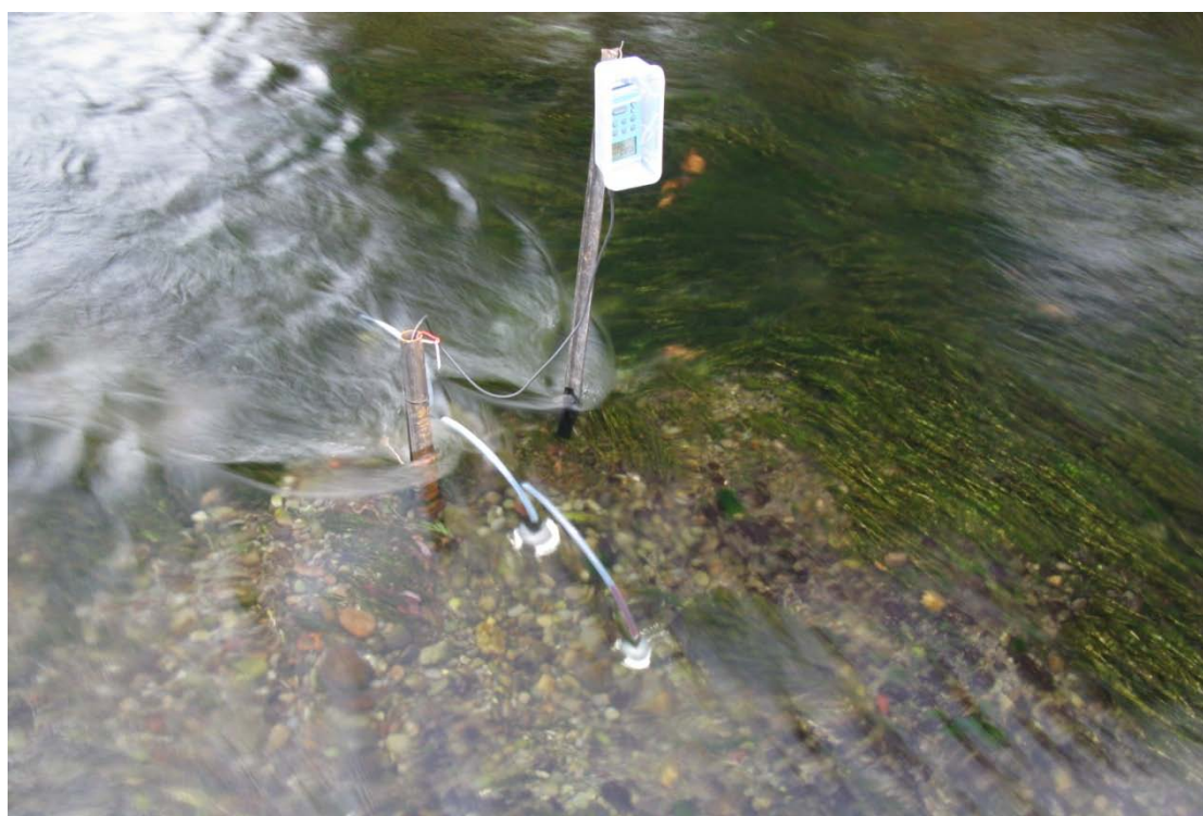
Figure 11. Use of the intragravel flow-monitoring technique. The logging conductivity meter is wired onto a waratah, with the probe inserted in the standpipe. The coloured saline solution is injected into the upstream IGDO probe.
